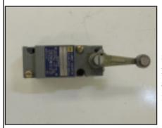
The limit switch already installed in my car, a Square D 9007 type limit switch with roller arm, has DPDT (double pole double throw) contacts. This means there were enough terminals to not only add the warning light, but to also wire it in such a way that the alarm and light could each be on their own fused circuit making them redundant to each other.
